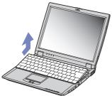
7 Lift the keyboard from the LCD display side and gently turn it over the touchpad. Be careful not to detach the cable (1) when lifting the keyboard.
